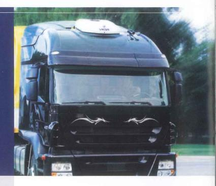
Kompressor II is a air-conditioning unit for the driver to rest when the vehicle is stationary.
